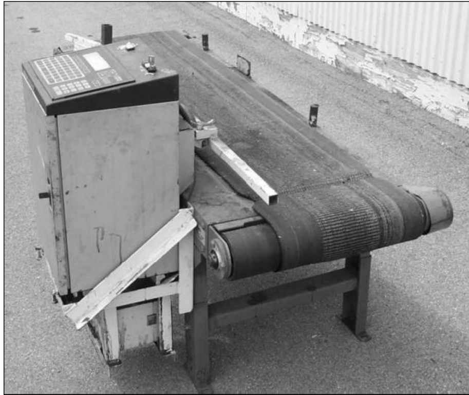
Fig.1. A flat belt conveyor with drive control
