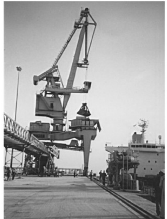
Fig. 8. 26 te level luffing kangaroo type portal crane in luff out and luff in positions
