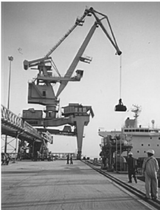
Fig. 8. 26 te level luffing kangaroo type portal crane in luff out and luff in positions
