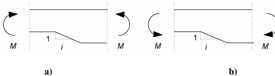
**Figure 6.14 Bending at a notch: a) with tensile stresses at the notch, b) with compressive stresses at the notch**
