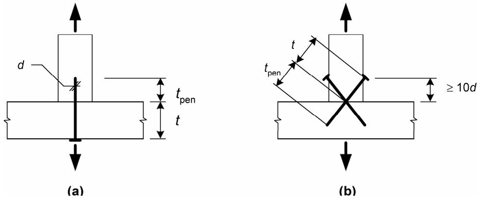
**Figure 8.8 (a) Nailing perpendicular to grain and (b) slant nailing**
