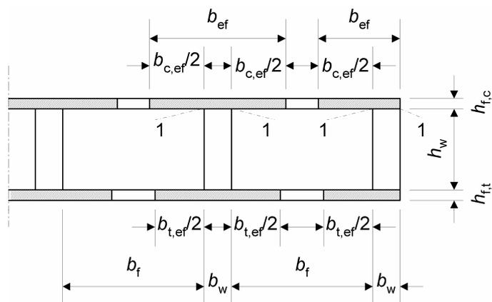
**Figure 9.2 Thin-flanged beam**
