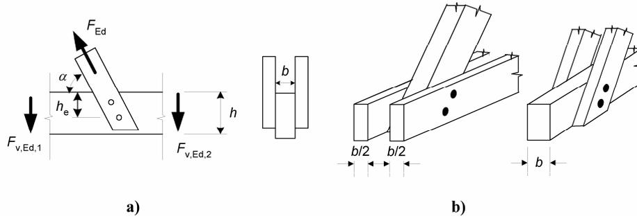
**Figure 8.1 Inclined force transmitted by a connection**
