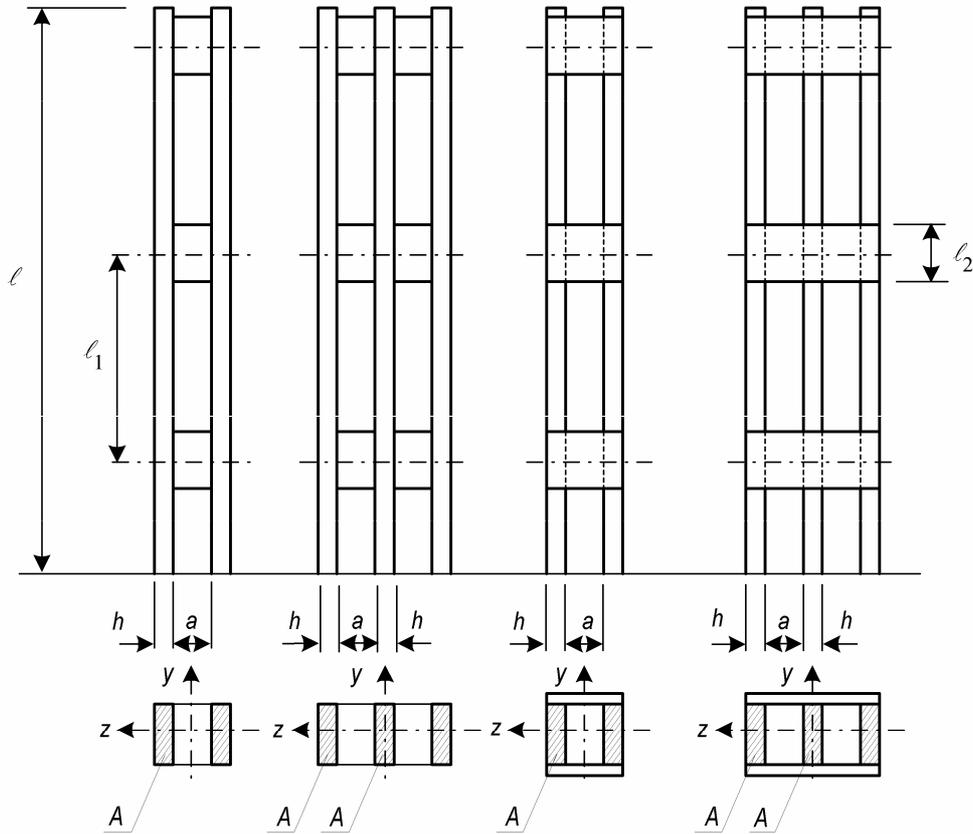
**Figure 11.1 – Spaced columns**
