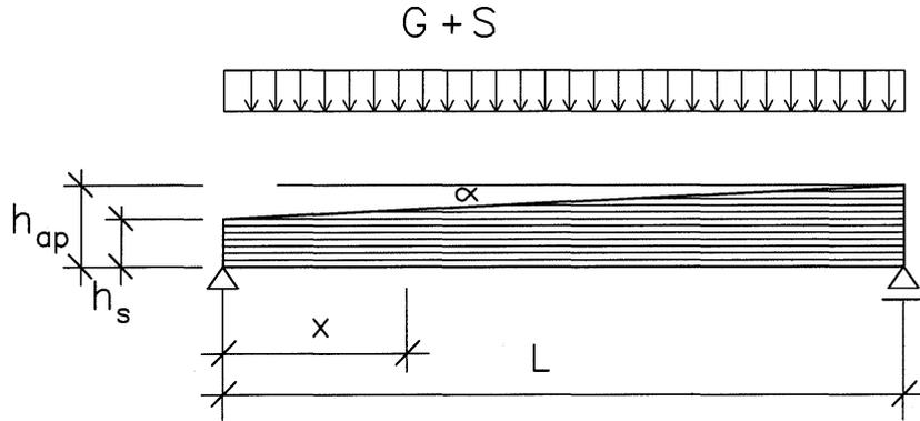
Fig. 10.1 Scheme of the single tapered beam
