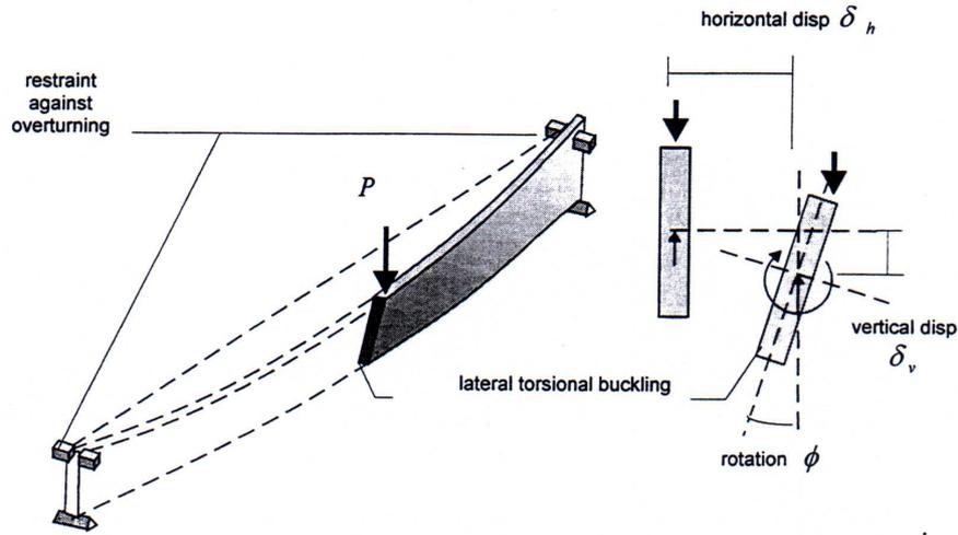
**Figure 6.11 Lateral-torsional buckling of simply supported beam**
