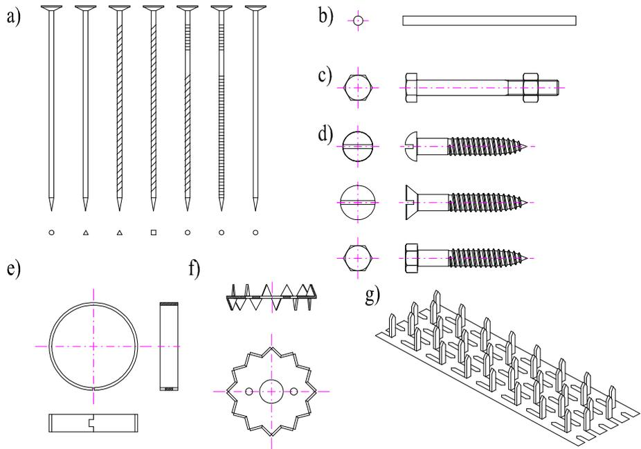
**Figure 8.1 Metal fasteners**
