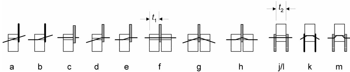
**Figure 8.3 Failure modes for steel-to-timer connections**
