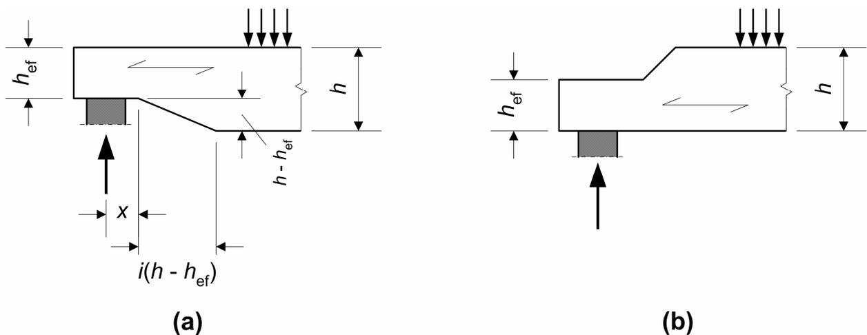
**Figure 6.15 End-notched beams**
