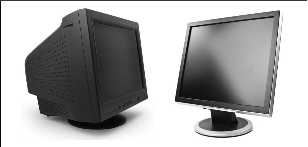
Figure 3-22, Comparison of CRT and LCD monitors
