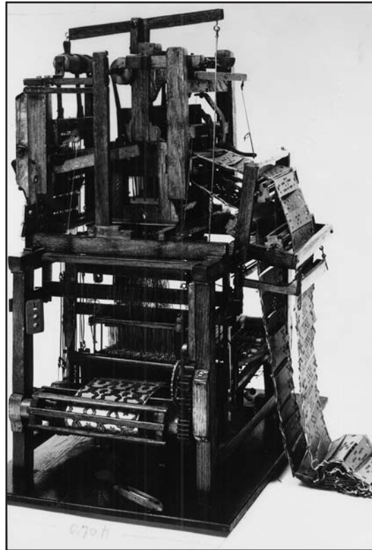
Figure 1-1, The Jacquard loom, using a string of punched cards that feed into the machine
