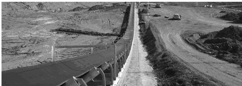
FIGURE 4.43 Overland troughed belt conveyor. Note that it can follow the general contour of the land.
