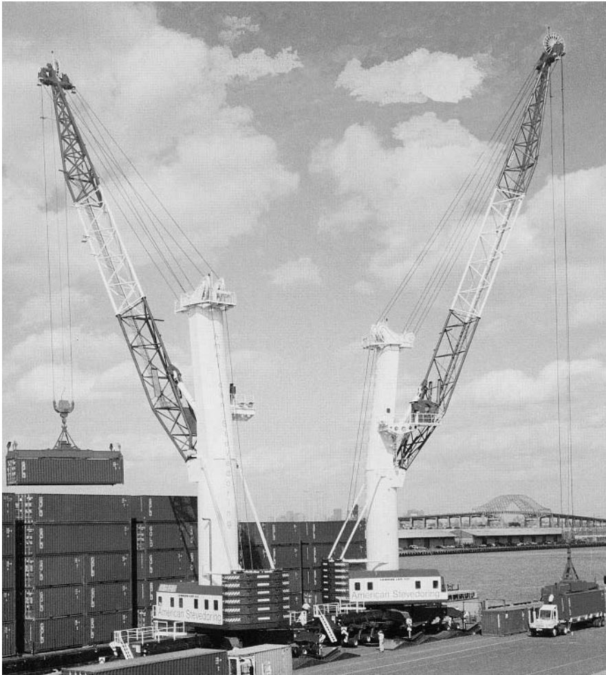
Fig. 1.1.6 100 t mobile ‘all-purpose’ crane
