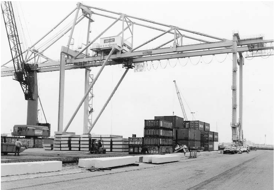
Fig. 10.2.3 Kalmar Container Crane with 70 m span
