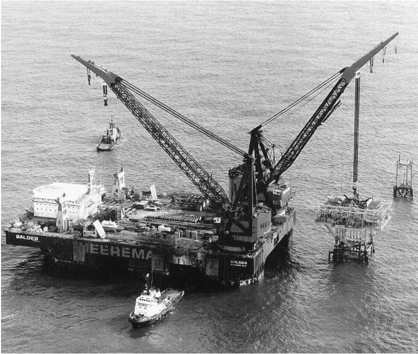
Fig. 1.3.9 Two offshore cranes; each for 4000 t (By courtesy of Heerema/IHC Gusto Eng. BV)
