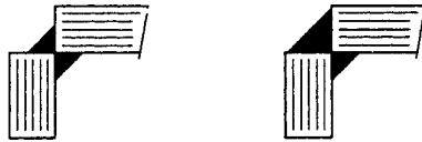
Fig. 7.2.3 Reduction of the sensitivity to lamellar tearing
