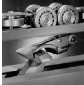
Fig. 6.2.13. An engagement mechanism between pusher and free trolley
