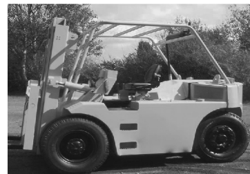
12 tons tilting mast diesel operated FLT
