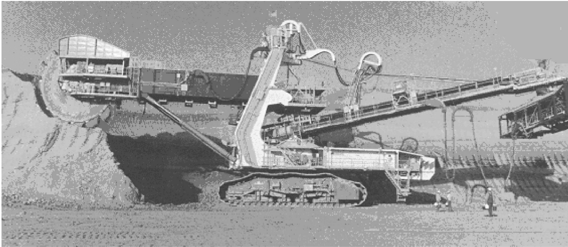
Fig. 9.2.1. Bucket wheel excavator, capacity 5000 m 3 /h
