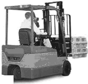
Battery operated FLT with single rear wheel
