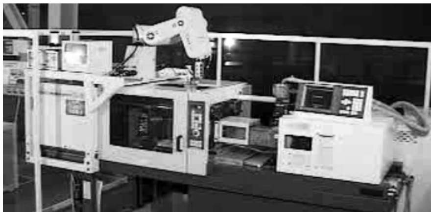
Fig. 10.3.1. Robot feeding component to CNC machine
