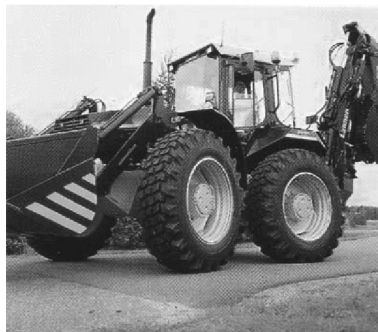
Tractor fitted with attachments on both ends
