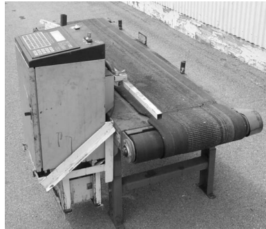
Fig. 6.1.1. A flat belt conveyor with drive control
