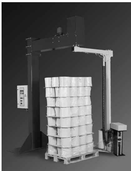
Fig. 3.6.4. Stretch wrapping machine. The pallet load is wrapped by a roll of film attached with rotating arm
