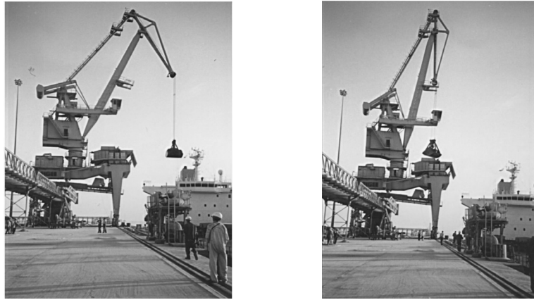
Fig. 8.5.16. 26 te level luffing kangaroo type portal crane in luff out and luff in positions
