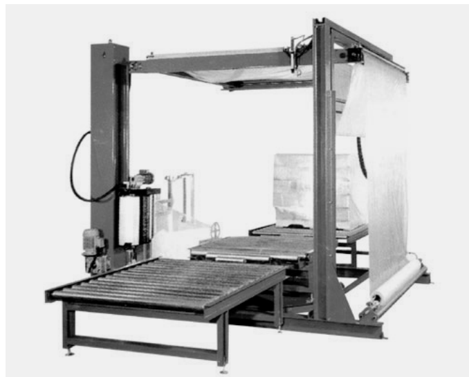
Fig. 3.6.5. Stretch wrapping machine for covering six sides of the load
