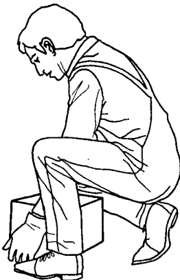
Fig. 36.1.1 Example of two-hand squat-lift method. Note straight back, spread feet, and the load is pulled between knees.
