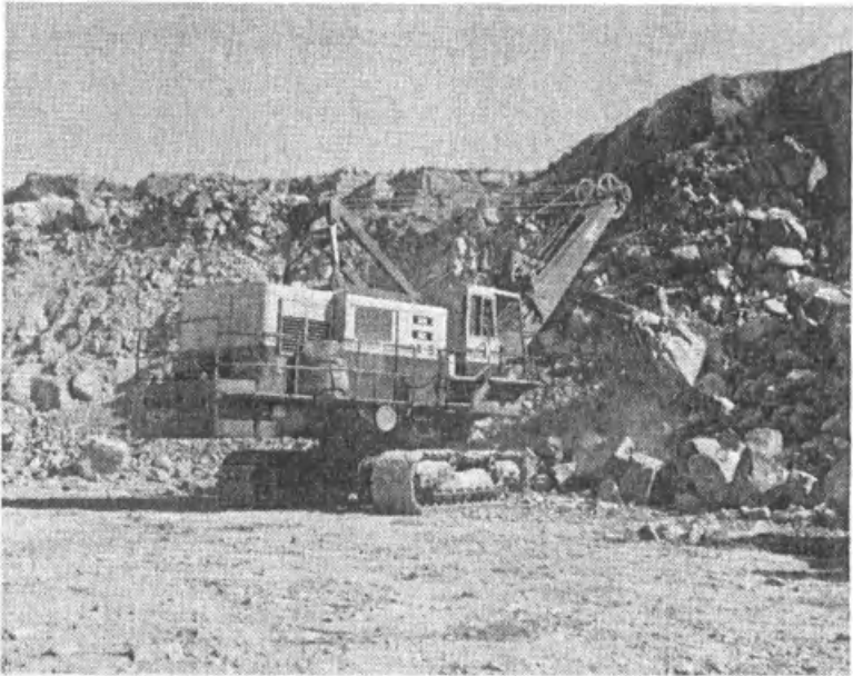
Fig. 31.3.1 Cyclic machine. Shovel operating in a granite rock quarry in Arkansas. Photo courtesy of Bucyrus—Erie.
