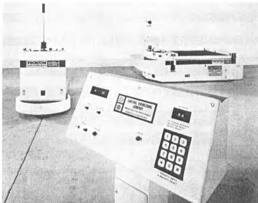
Fig. 8.2.16 Manual entry panel performs unattended load dispatch. (Courtesy of Control Engineering Co., Affiliate of Jervis B. Webb Co.)
