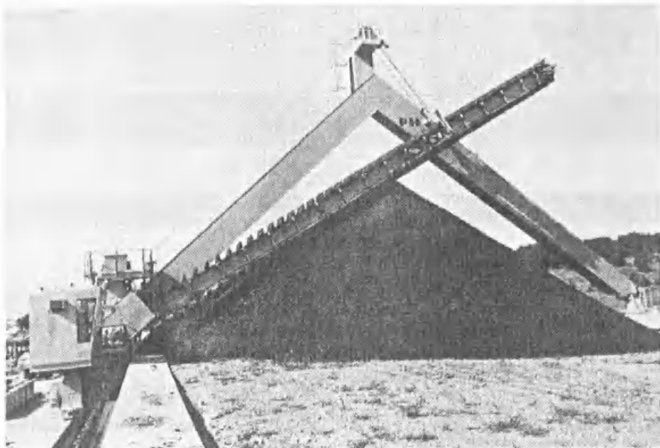
Fig. 31.3.2 Full portal scraper. This portal type scraper is a unique stacker/reclaimer. It operates on a coal stockpile for a cement plant in Texas. Photo courtesy of PHB Weserhutte A G.
