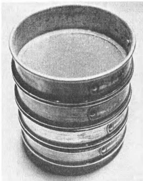
Fig. 20.2.5 Testing sieves (range of 24, 40, 60, 100, 200, and 350 mesh) used to classify materials.
