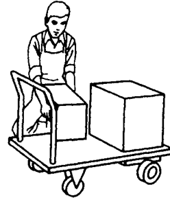
2. PLACE LOADS PROPERLY on four-wheeled trucks, to avoid tipping, ensure steering ease.
