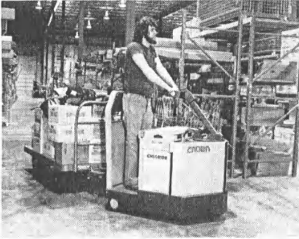
Fig. 7.2.5 A walkie-rider at work in an order-picking application. (Courtesy Crown Controls Corp.)
