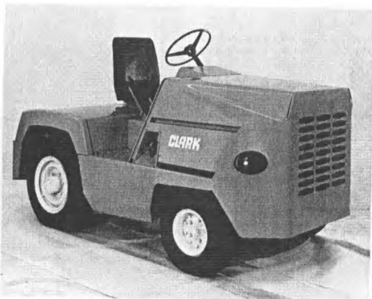
Fig. 7.2.4 Typical internal combustion-powered 5000 lb (22, 241 N) drawbar pull tow tractor. (Courtesy Clark Equipment Co.)
