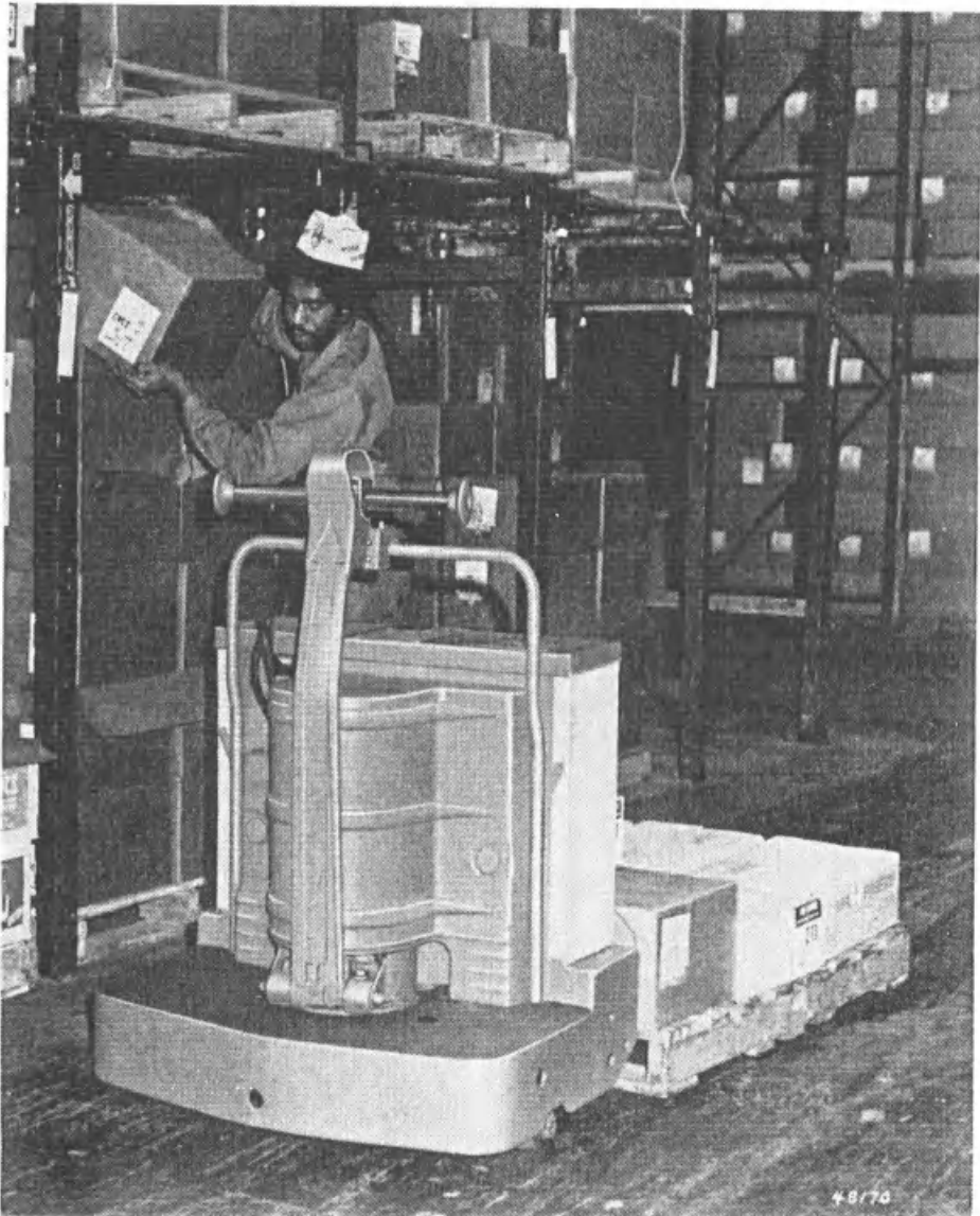
Fig. 7.1.2 Walkie/rider low-lift pallet truck. Note the lift/lower control on bar and operator riding the platform.
