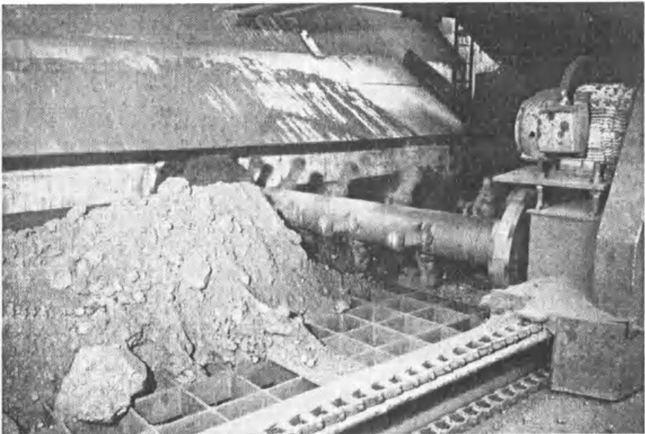
Fig. 33.1.5 Lump breaker on grizzly beneath rotary car dumper.
