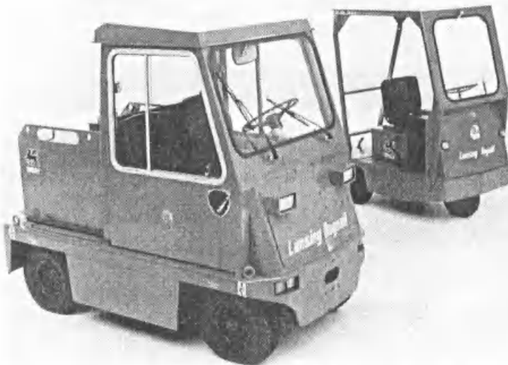
Fig. 7.2.2 Typical sit-down rider electric tow tractor. (Courtesy Lansing Bagnall Corp.)
