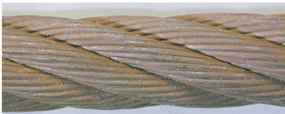
Figure H.1 — Beginning of surface oxidation, can be wiped clean, superficial — Rating: 0 % towards discard
