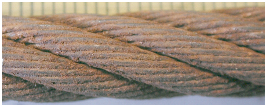
Figure H.1 — Beginning of surface oxidation, can be wiped clean, superficial — Rating: 0 % towards discard
